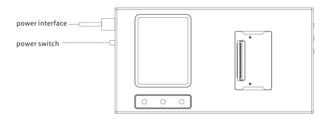
Shutdown:Switch the 'Power Switch' to the 'OFF' state to turn off the power supply of the M830 test box, and then unplug the power cord.
