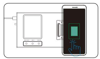
**STEP3:**Level 1 pressure test Gently press with your fingers, and the inner frame will display green, indicating a level 1 pressure test
