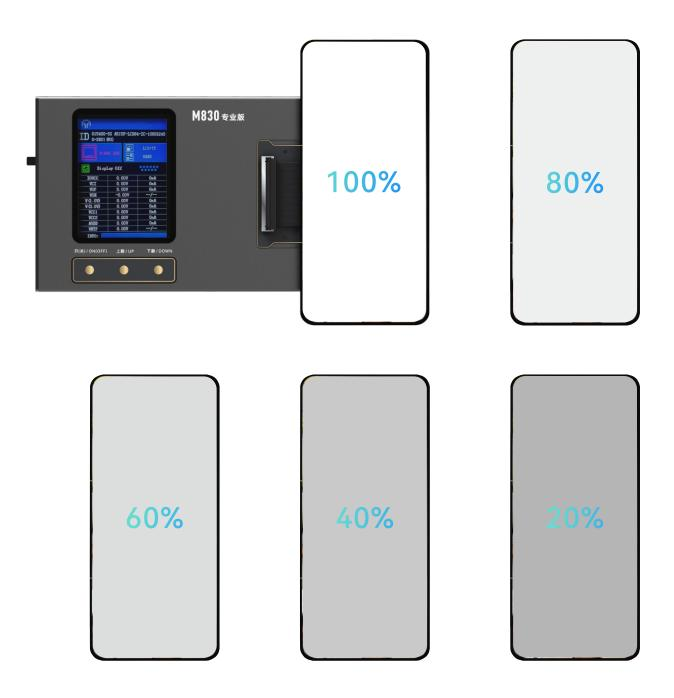
Short press the K1 key to activate the brightness cycle test function
