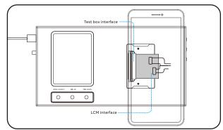
**STEP1:**'Test screen' connectionThe "screen to be tested" corresponds to the transfer board and transferConnect the cable to the M830 test box.
