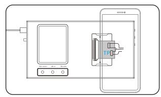
**STEP1:**'Test screen' connection The TP interface of the "screen to be tested" corresponds to the adapter board and is connected to the adapter cable and M830 test box.
