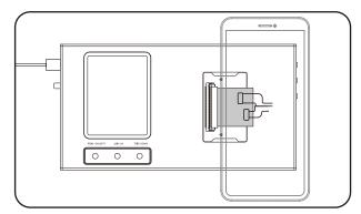
**STEP1:**The 'screen to be tested' is lit The 'screen to be tested' is connected to M830 and lit. Click "Flip Up, Flip Down" to switch screens normally.
