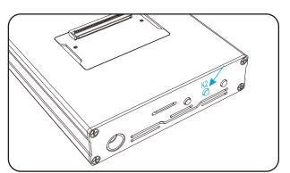
**STEP2:**Read the original screen color program Long press the K2 key to switch to the True TONE function. Click the 'flip up' button to read the original color code.
