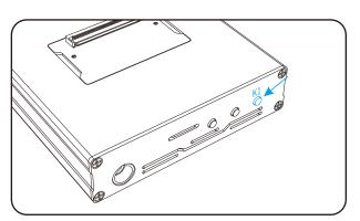
**STEP2:**Identification program If the automatic recognition cable is incorrect or not recognized, click the "K1" button to identify the model.
