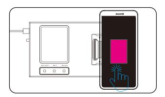
**STEP4:**Level 2 pressure sensing test Finger pressure increases, and the inner frame displays red, indicating a level 2 pressure test
